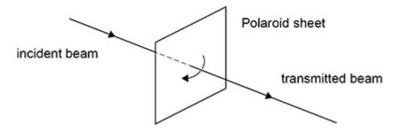
The Polaroid sheet is rotated about the beam by 90° and the intensity of the transmitted beam decreases to zero.
