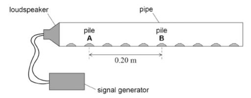
The distance between pile **A** and pile **B** is 0.20 m.
