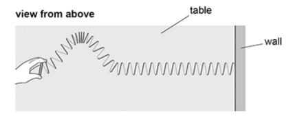
The free end of the spring is quickly moved to one side and then back to the centre, creating a pulse.
